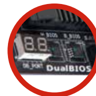
Gigabyte has equipped the board with a pair of physical BIOS ROMs.
